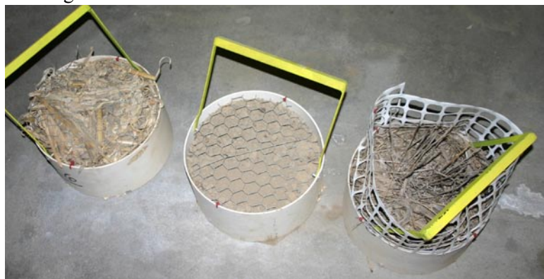
Above: These mini-lysimeters are used to measure water evaporation from the soil at the SWREC, Garden City, Kan. From left includes corn stalk no-till, bare soil, and wheat stalk no-till. By comparing the no-till stalks to the bare soil, researchers can determine which type of ground cover loses the least water through evaporation. Right: A bare soil mini-lysimeter in the crop field at the SWREC.
