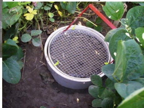
Above: These mini-lysimeters are used to measure water evaporation from the soil at the SWREC, Garden City, Kan. From left includes corn stalk no-till, bare soil, and wheat stalk no-till. By comparing the no-till stalks to the bare soil, researchers can determine which type of ground cover loses the least water through evaporation. Right: A bare soil mini-lysimeter in the crop field at the SWREC.
