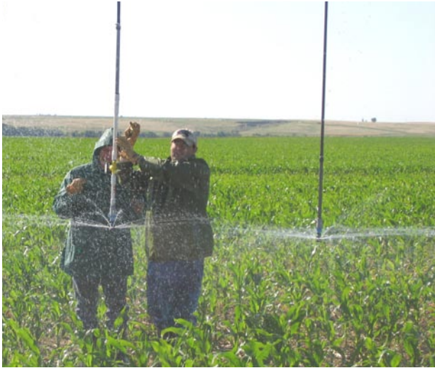
During field evaluations, water flow and pressure of nozzles also are checked. This requires the sprinkler to be irrigating, resulting in evaluators getting very wet.
